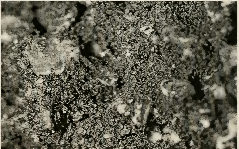
Figure 4.7 Photomicrograph of surface of sample 1.04-1 from the living room. The original layer is coarsely textured and the various pigments are visible. 50X.
